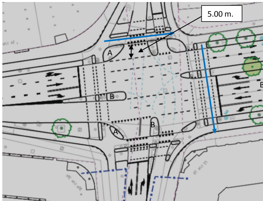
Fig. 6.7 Segregated design at intersection with one-way cycle tracks
