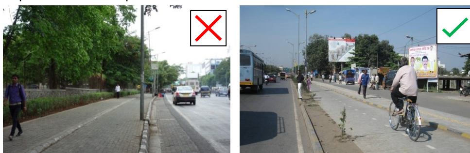
Fig. 4.4 Raised adjacent cycle track in Pune
