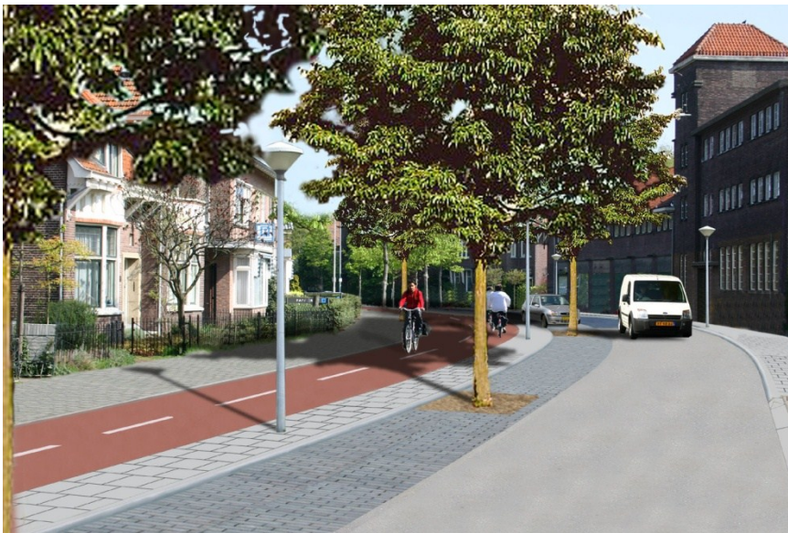
Fig. 2.6 One-way, one lane road with two-way cycle track (this road used to have two traffic lanes)
