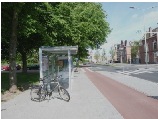
Fig. 7.10 Bus shelter behind the cycle track and Island for bus stop
