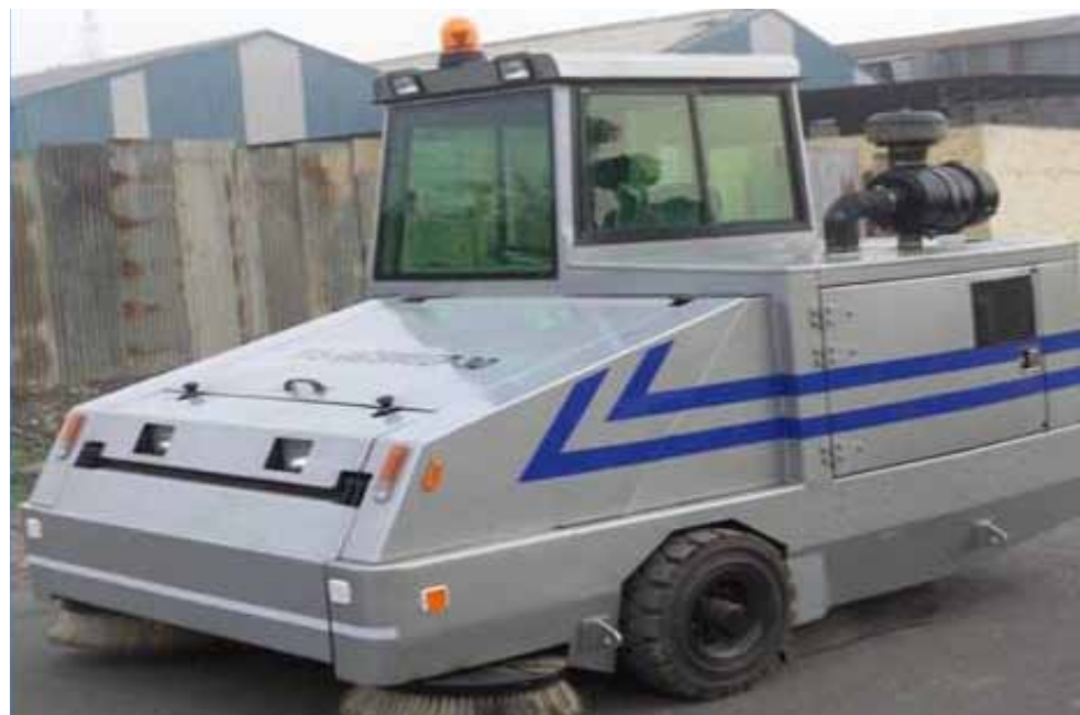
Figure 2.20: Self-propelled road sweeping machine 28
