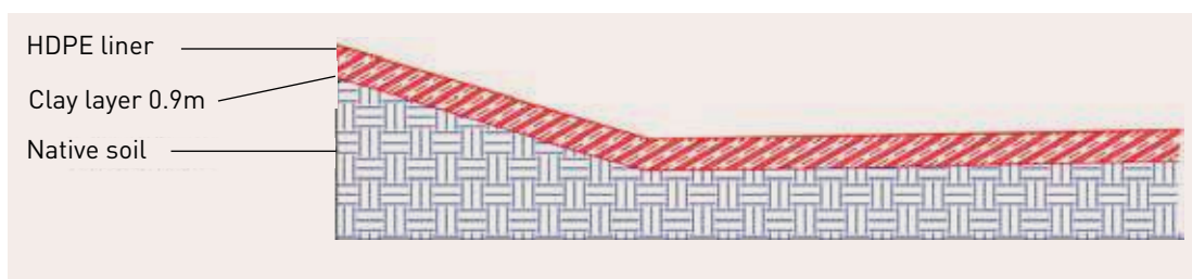
Figure 4.7: Placement of the High density Polyethylene Liner over the Clay Liner 10
