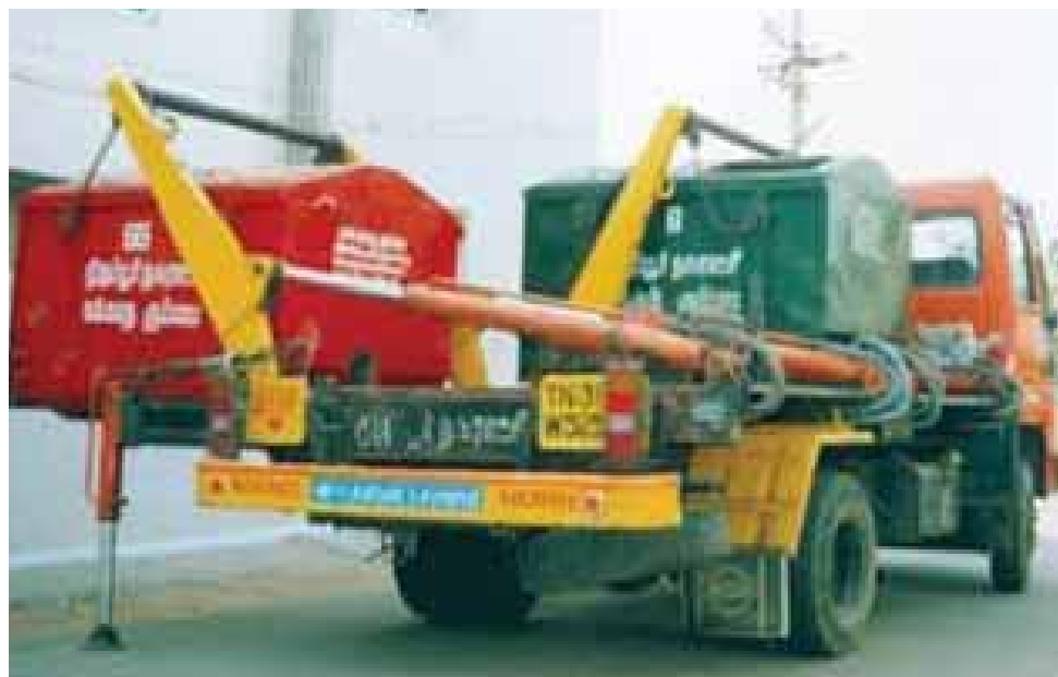
Figure 2.13: Skip Truck (Dumper Placer Machines) 17
