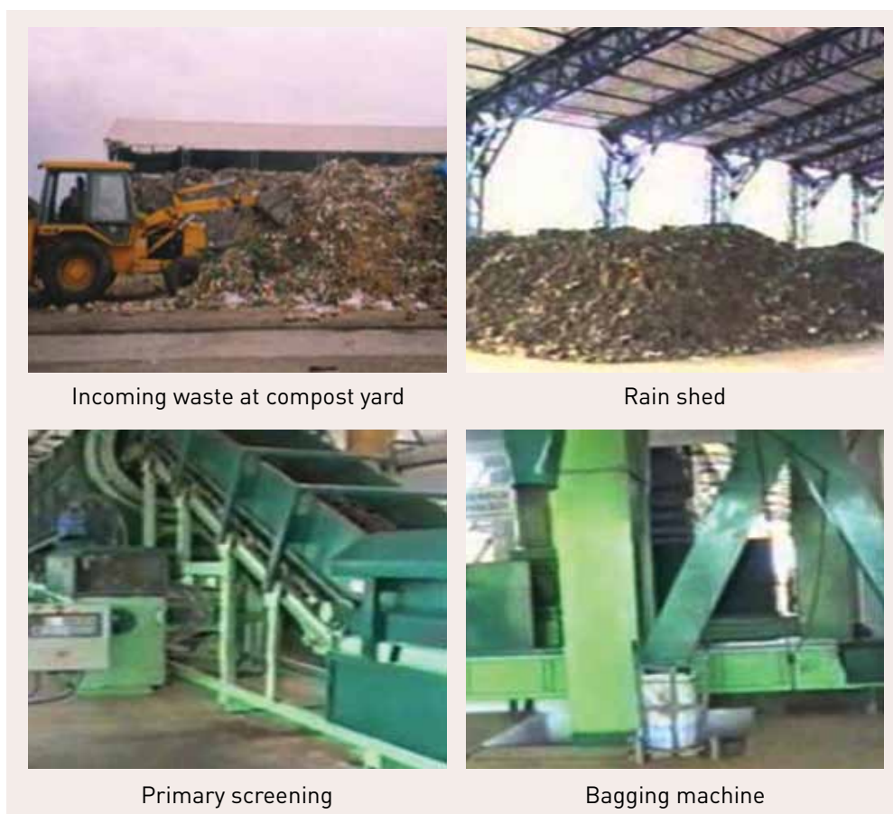
Figure 3.15: Unit operations in windrow composting 20
