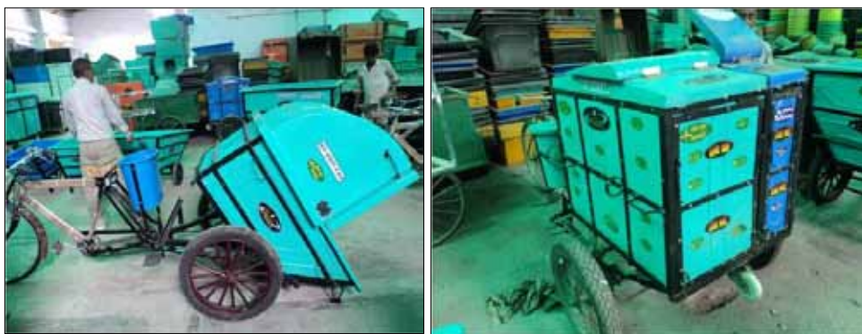
Figure 2.9: Tricycle with Hydraulic Tipping Container 14
