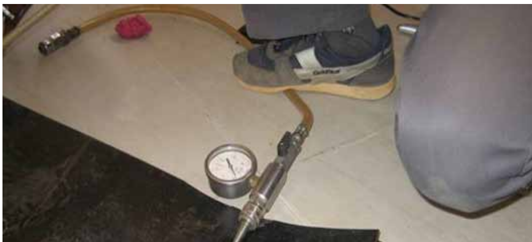
Figure 4.17: Proof of welding seams 21
