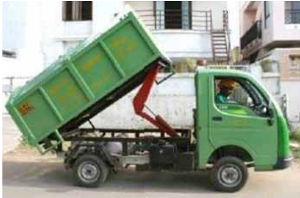
Figure 2.10: Mini Truck with Hydraulic Container
