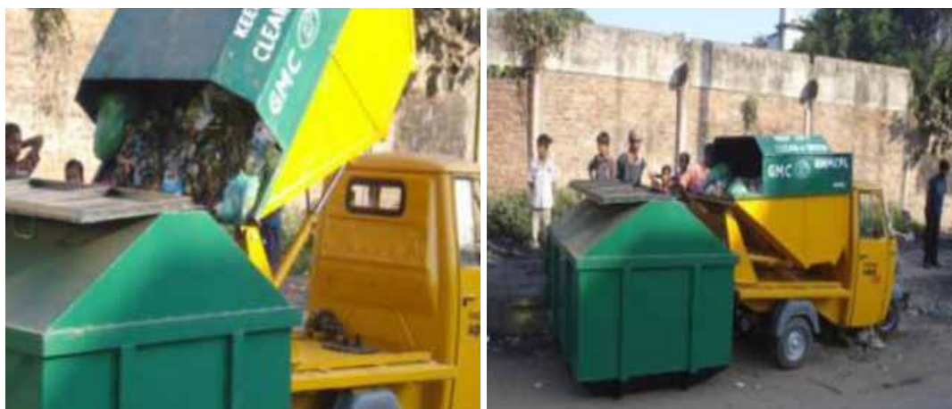
Figure 2.12: Synchronised Primary Collection and Secondary Storage 16
