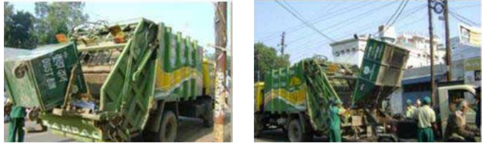
Figure 2.15: Transfer of Waste from Secondary Collection Bins to Refuse Compactor 19
