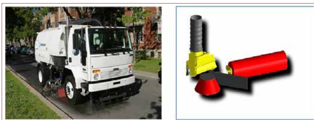
Figure 2.19: Vacuum Sweeper and Vacuum Nozzle 27
