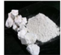
This involves addition of alkaline compounds like lime to the sludge which in turn increases the pH thereby inhibiting microbial activity.
