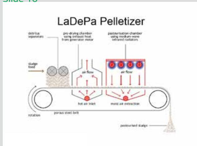
Schematic showing the working of a LaDePa pelletizer
