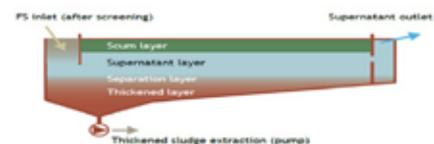
Gravity separation is employed for separation of the heavy solids and the supernatant liquid. Settling-thickening tank works on this principle.
