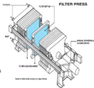
Construction and working of a plate and frame filter press for mechanical dewatering. For more information refer to FSM Book (Strande, Ronteltap, & Brdjanovic, 2014).
