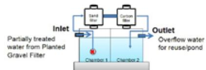
SCF is used to remove the turbidity, TSS colour and odour. A schematic explaining the working of sand and carbon filter is shown in the slide.
