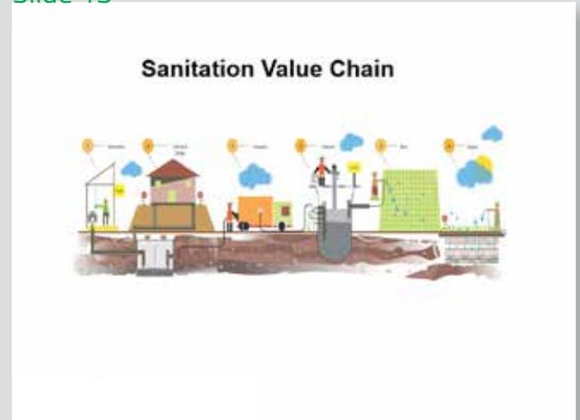
The sanitation value chain is a diagrammatic representation of the movement of faeces from generation to disposal. It has six components:
