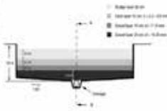
Sludge drying beds are mainly used for dewatering of stabilized sludge.
