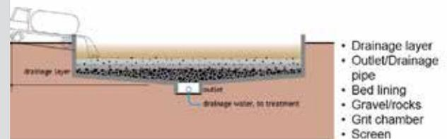
Figure representing the various components of an unplanted drying bed.
