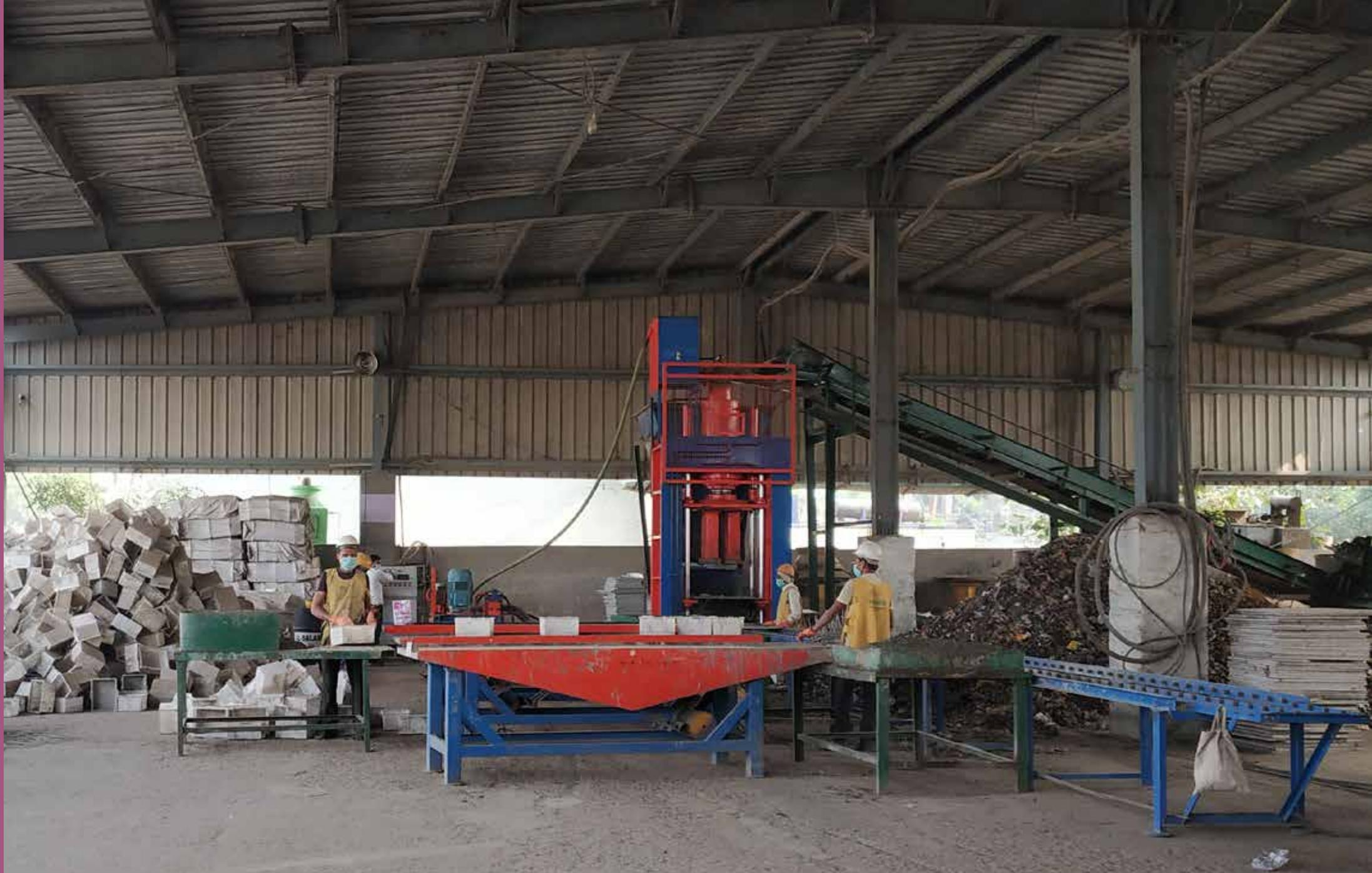
Dry Waste Compressed to make RDF Block
