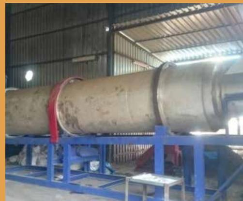
Dryer Machine used for composting
