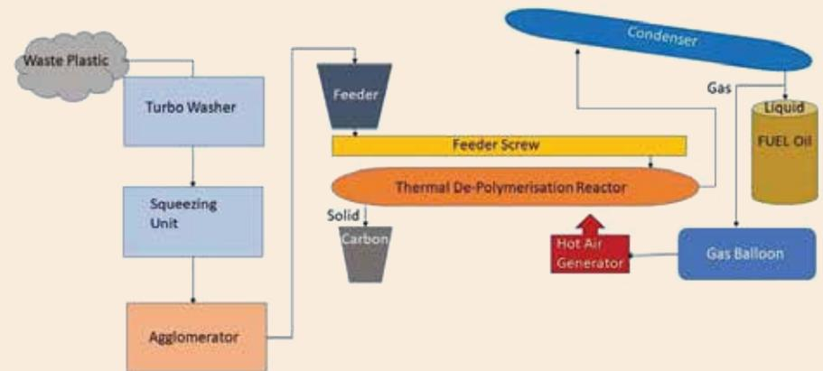
The plant has capacity to process 4 MT of plastic with an efficiency of loading of 400 kg per hour. In this plant, only good quality of plastic is processed for fuel production while the remaining is used as RDF. The entire process finishes in 10 hour. The output is FO grade oil which is used in small industrial furnaces. There is 40-45% oil recovery per day which is equivalent to 1500-1800 litre per day. The generated gas is used in
