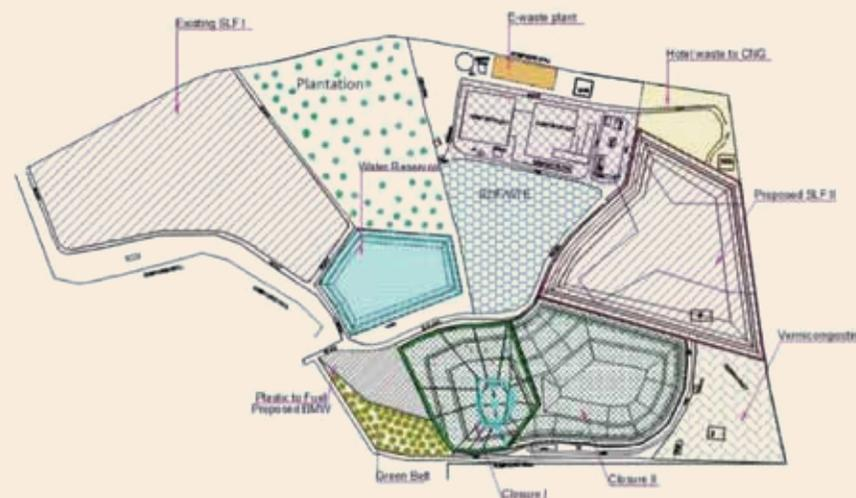
The site has a mechanical composting plant of a capacity of 450 MT per day, a vermicomposting plant of a capacity of 20 MT per day and a plastic-to-fuel plant with a capacity of 5 MT per day. This centralized processing unit has the following facilities:
