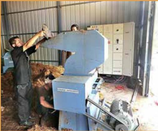
Shredding of Cocount at Cocount Waste Processing Plant
