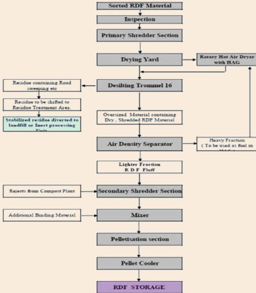
The plant produces 10-20 MT G1 grade, 20-30 MT G2 grade and remaining 100 MT is of G3 or SCF grade.
