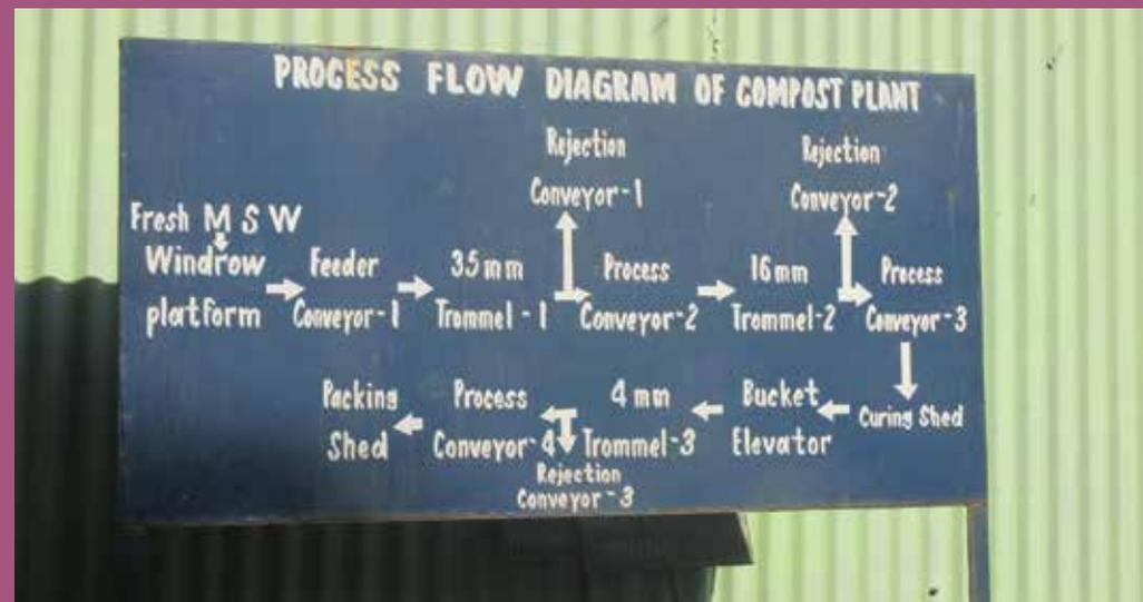
Process Flow Diagram of Compost Plant
