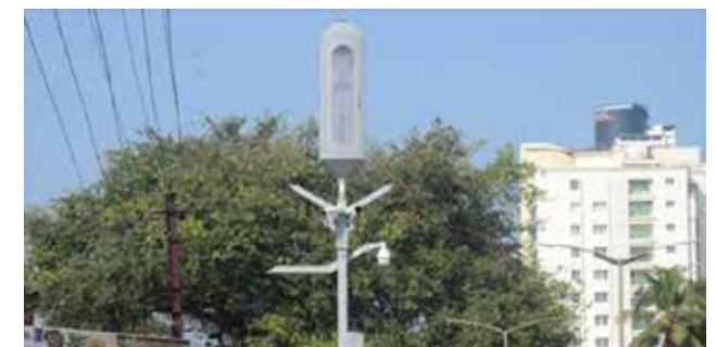
Figure 14 Smart Pole with 4 fixed focal length cameras, one PTZ, and a digital screen showing information related to AQI (Source Daijiworld Media Network - Mangaluru (SP))
