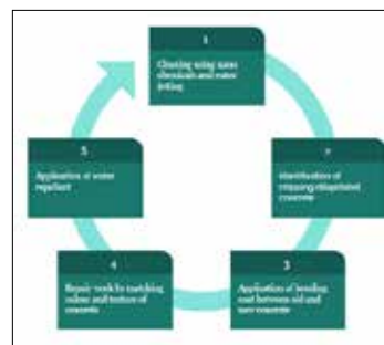
Figure 2.16: The process of restoring exposed concrete edifices; Source: Author
