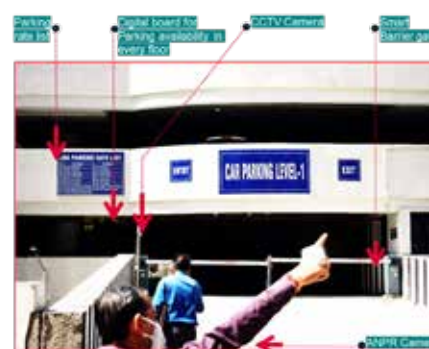
Figure 2.4: MLCP Project with Smart features
