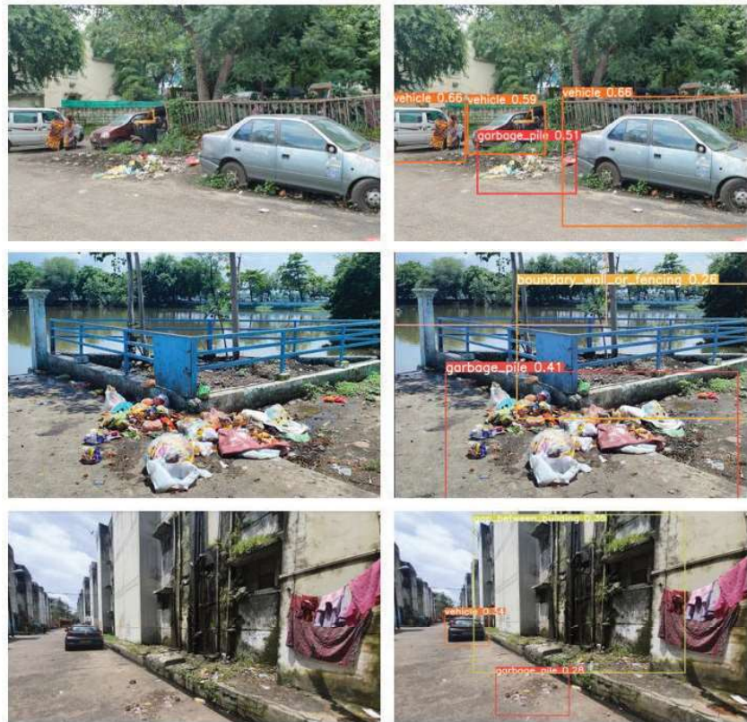
IMPROV IMPROV's AI/ML-based multi-layer object detection and classification model for identifying garbage vulnerable spots
