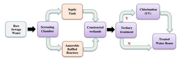
Figure 11: Integrated treatment set up with CWs
