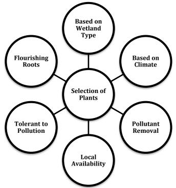
Figure 16: Factors to be considered for selection of plants for constructed wetlands
