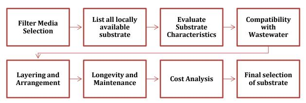
Figure 13: Indicative steps for substrate selection for constructed wetlands
