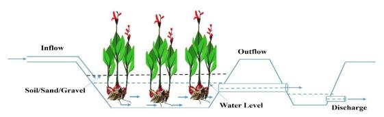
Figure 3: Basic design configuration of horizontal flow constructed wetlands
