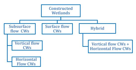
Figure 1: General classification of Constructed wetlands
