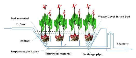
Figure 2: Basic design configuration of vertical flow constructed wetlands
