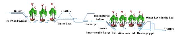
Figure 5: Basic design configuration of hybrid constructed wetlands
