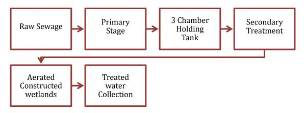
Figure: Process flow diagram
