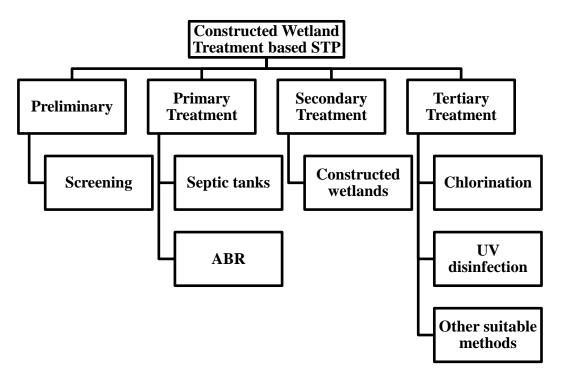
Figure 9: Process flow of CWs based STPs
