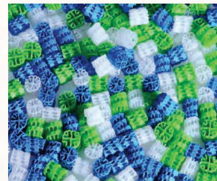
The carrier material in MBBR system
