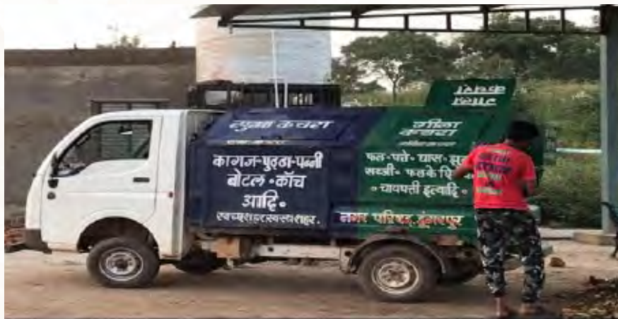
Waste collection vehicles with separate compartments for segregated collection
