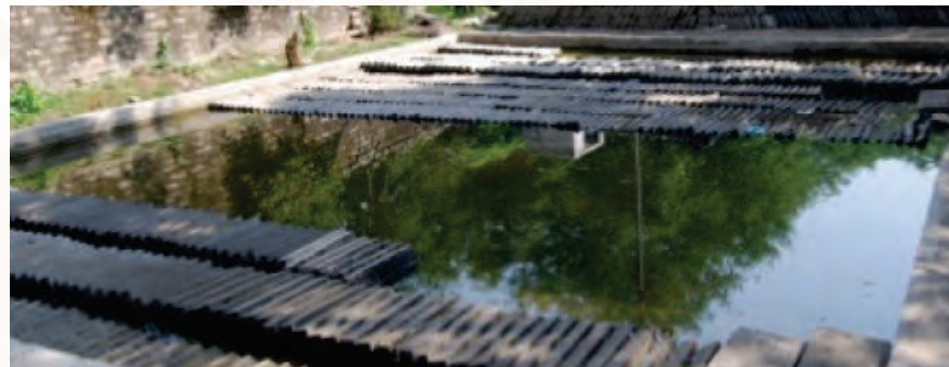
The Concrete tiles are put in pond for curing
