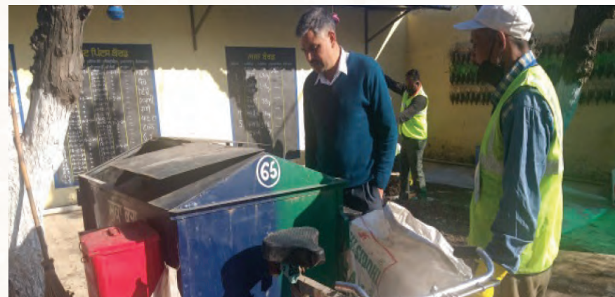
Separate compartments in waste collection vehicles for segregated collection
