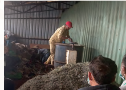
Non-recyclable plastic shredded with the help of shredding machine
