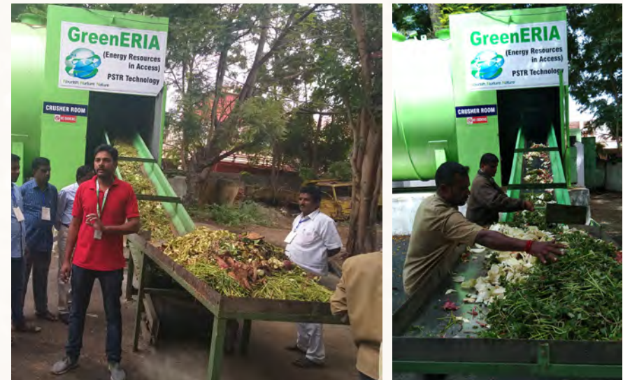
Organic waste passed to the shredded through the conveyor belt
