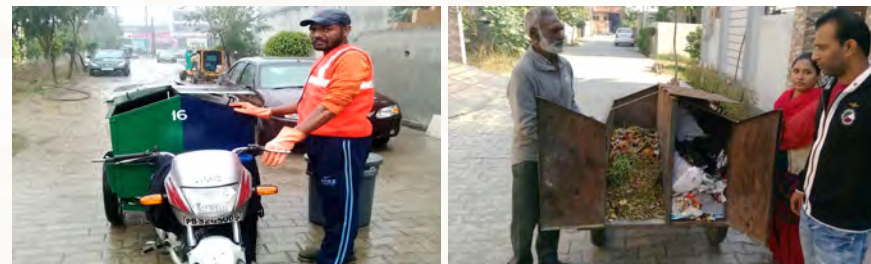
Waste collection in tricycles with compartments for segregated waste
