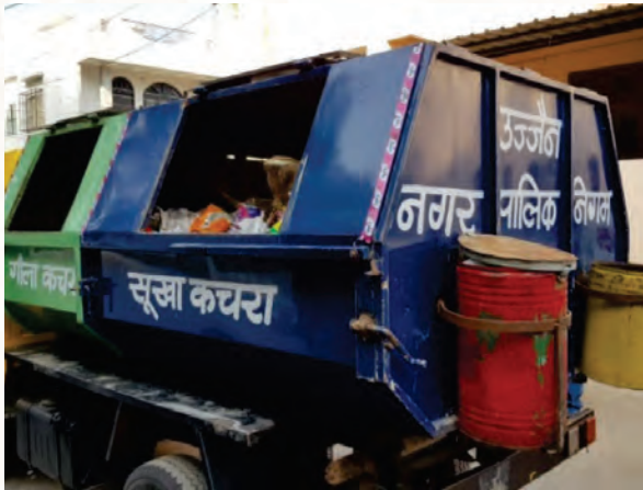
Segregated Door to Door Collection. Besides separate compartments for dry and wet waste, the garbage collection vehicle also has separate bins for Domestic hazardous waste. (Yellow bin - Sanitary waste and Red bin for sharp items, razer blades, glass,etc.)
