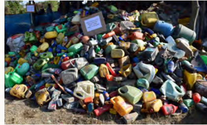
Segregated HDPE grade plastic
