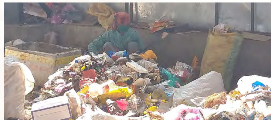
Waste being further segregated at the MRF
