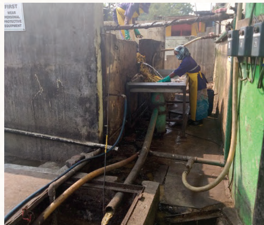
Crushing of waste to form a slurry
