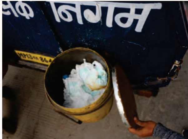
Segregated Door to Door Collection. Besides separate compartments for dry and wet waste, the garbage collection vehicle also has separate bins for Domestic hazardous waste. (Yellow bin - Sanitary waste and Red bin for sharp items, razer blades, glass,etc.)
