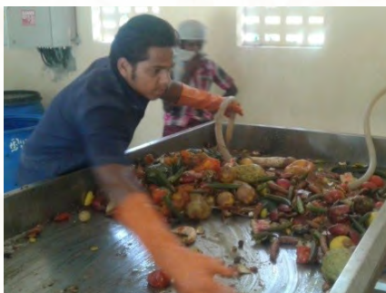
Making slurry to feed into digester
