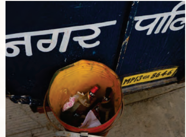
Segregated Door to Door Collection. Besides separate compartments for dry and wet waste, the garbage collection vehicle also has separate bins for Domestic hazardous waste. (Yellow bin - Sanitary waste and Red bin for sharp items, razer blades, glass,etc.)
