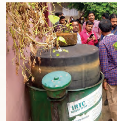
Portable Biogas Plant
