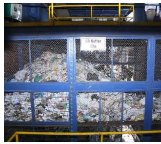
(c) Segregated waste receiving chamber
