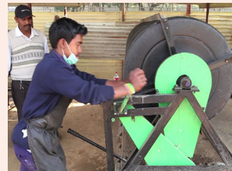
Figure 4.60: Rotary Drum Composting
