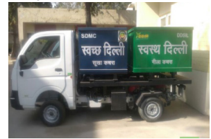
(c) Auto tipper with separate containers for collection of Dry and Wet Waste
