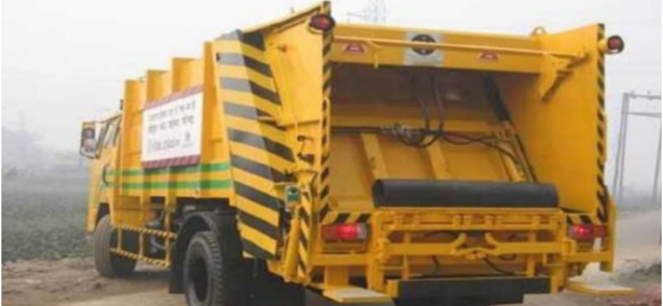
Figure 4.21: Refuse Compactor Truck
