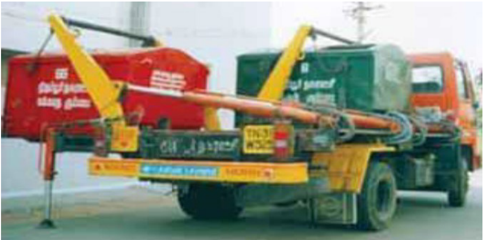
Figure 4.20: Skip Truck (Dumper Placer Machines)
