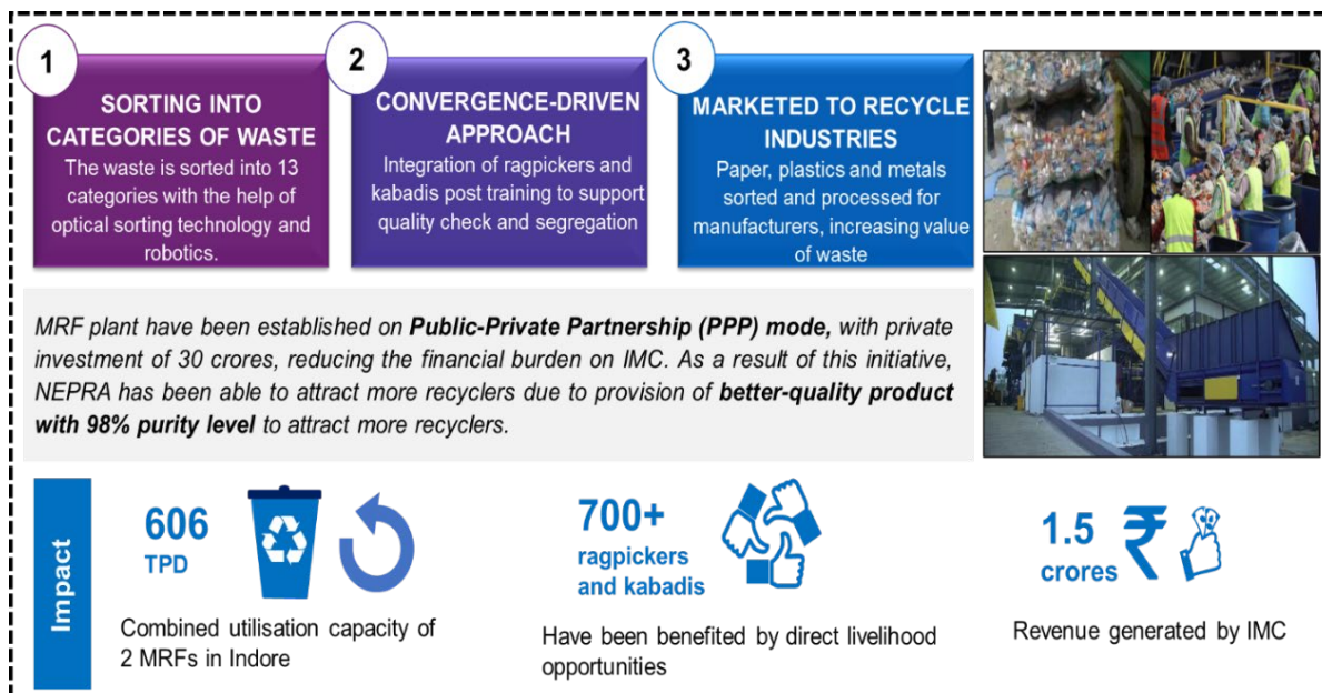
Figure 8: Automated MRF at Indore
