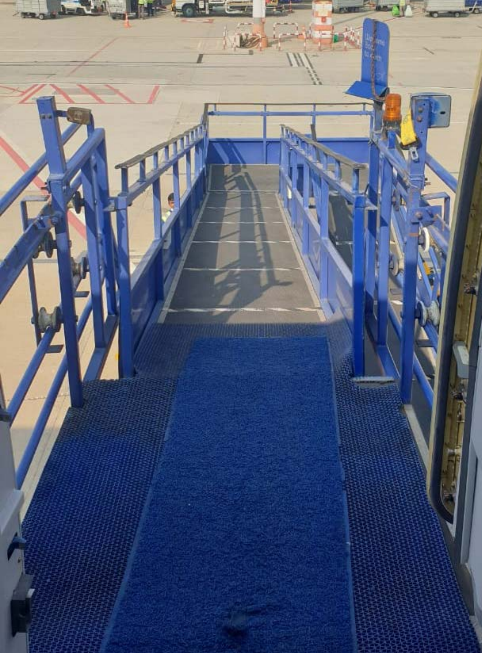
Image 6.30 Accessible ramps for aircraft boarding
