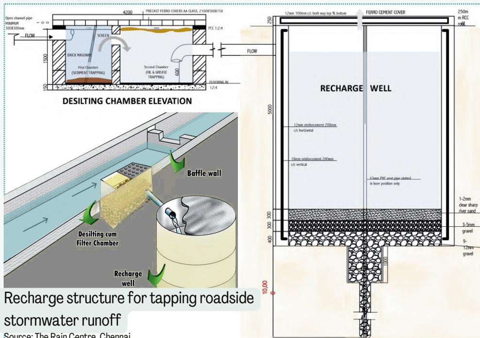
Recharge structure for tapping roadside stormwater runoff
