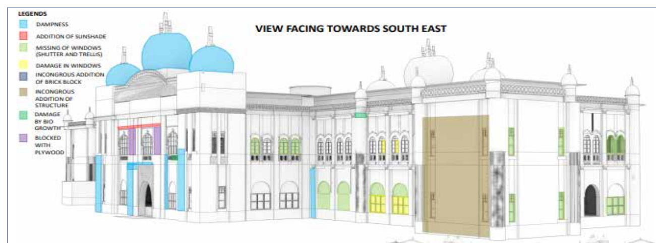
Figure 4: View of existing structural condition of the collectorate building
