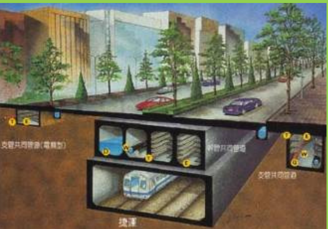
Rectangular CUD with or without partition (accessible through Manholes)
