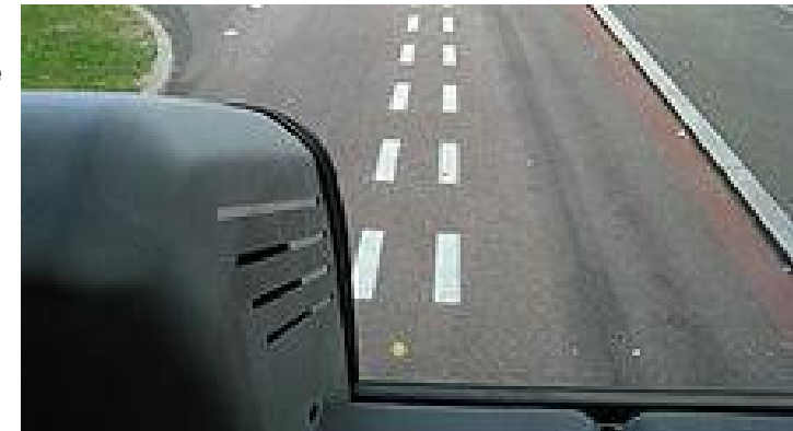
Optical guiding device on bus in Rouen,
