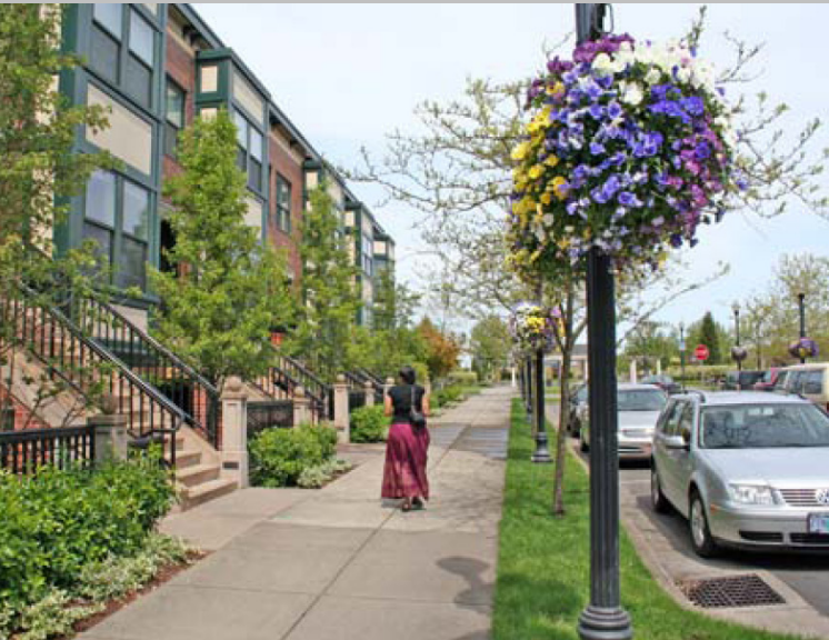
Continuous planting zones are suitable for areas where pedestrian volumes are less and they need to be contained within the walking zone.
