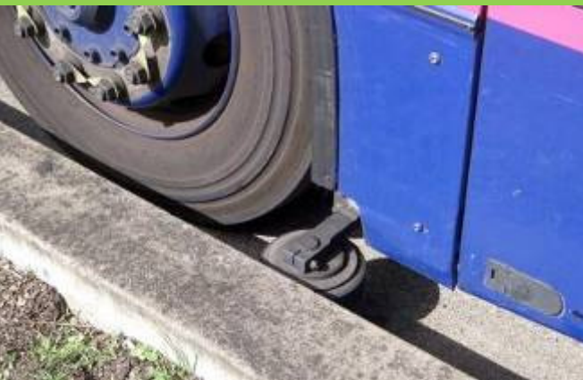
View of kerb Guide wheel
