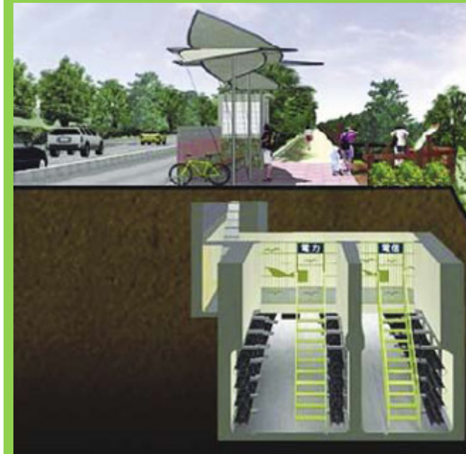
Sketch of a Fully accessible CUD with respect to the Street above.
