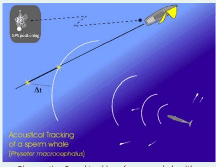
Bioacoustics: Sound tracking of a sperm whale with a dipole array
