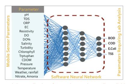
Real-time application of a neural network to easily available parameters, for predicting complex water quality indicators
