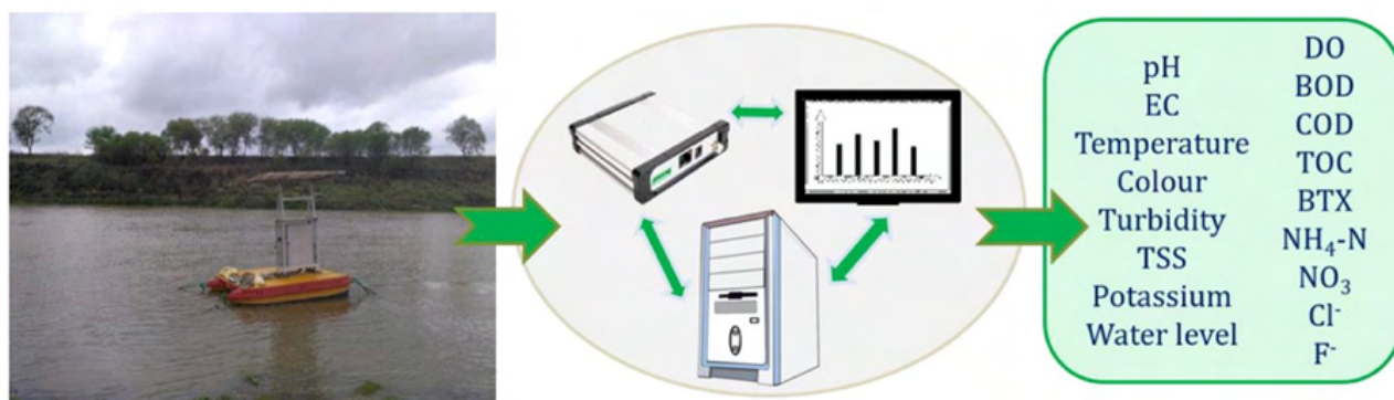
Figure 27: Parameters measured by real-time water quality monitoring stations (Source: NMCG)
