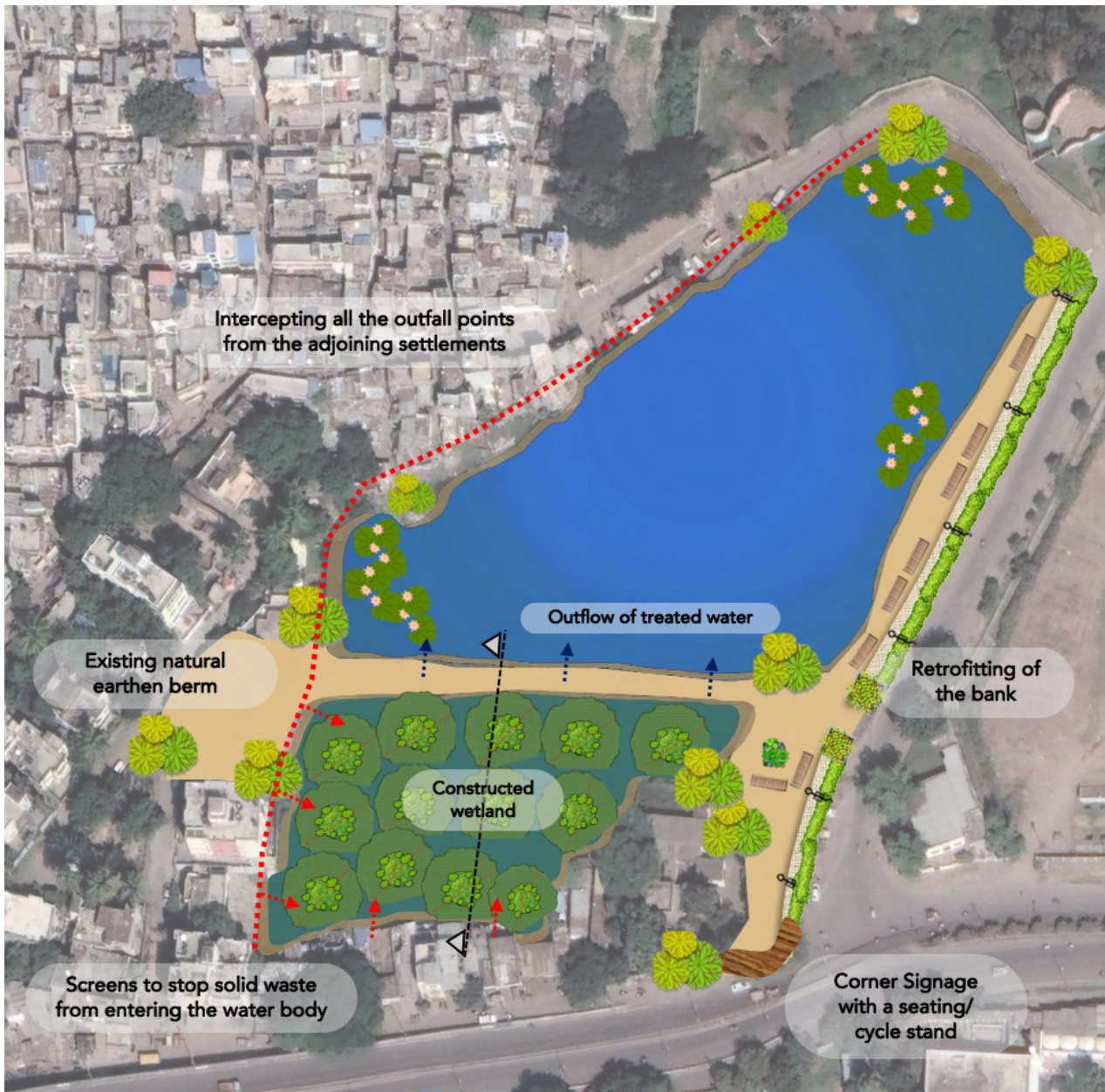
Figure 37: Schematic diagram showing rejuvenation of Kamal Talao
