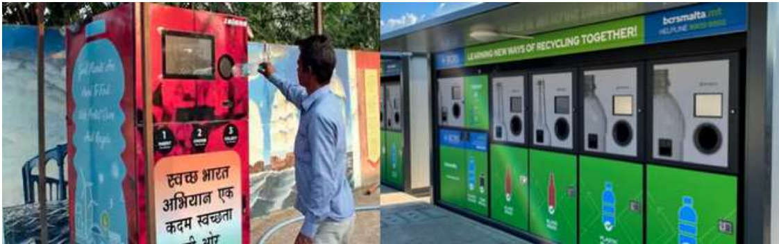
Image 38: Reverse vending machine sample models that can be used along Sarayu ghats.
